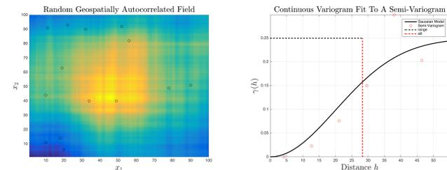
**a:** A geospatially autocorrelated field with samples taken at the locations marked. **b:** A Variogram fit from a discrete variogram (Eq. 2).
